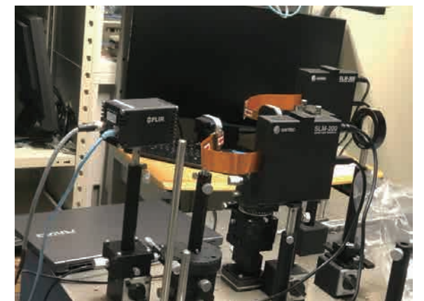
An optical system that uses two Santec SLM-200s simultaneously to control the amplitude and phase of light. This will enable the creation of holographic TVs.
