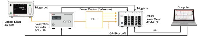
IL / PDL measurement setup with the polarization controller PCU-110 and the power meter MPM-210H
